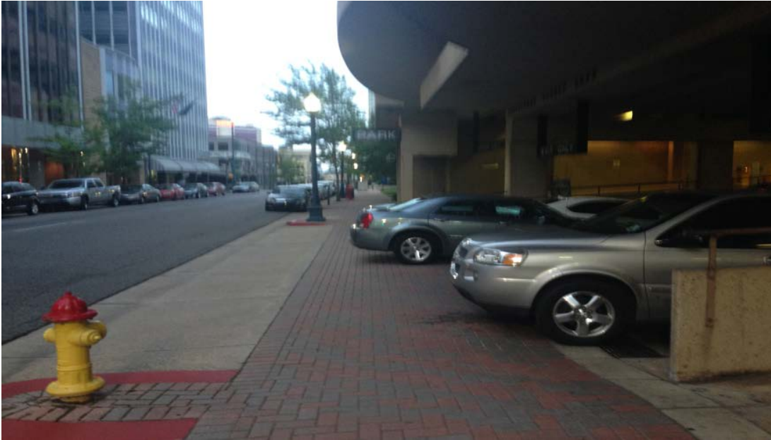
Private off-street garage parking cars on the sidewalk in violation of the Americans with Disabilities Act which require a minimum of 4' of level sidewalk surface be kept clear. Photo Credit: Jeremy Nelson
